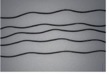
Long Wave Filaments Amplitude: 0.10 – 0.25 mm Wavelength: 3.50 – 5.50 mm
