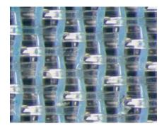
**High pressure cleaning test**Forming fabric from DuraFil® monofilament (blue threads). The monofilaments exhibit no damage whatever.
